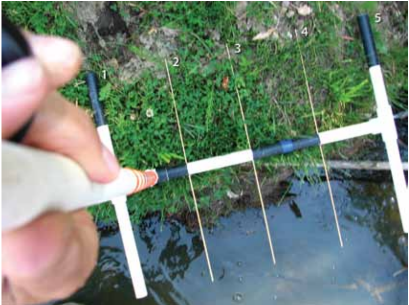
Figure D6. Lines 1, 2, and 4 intersect streambank alteration. A “3” is recorded.
