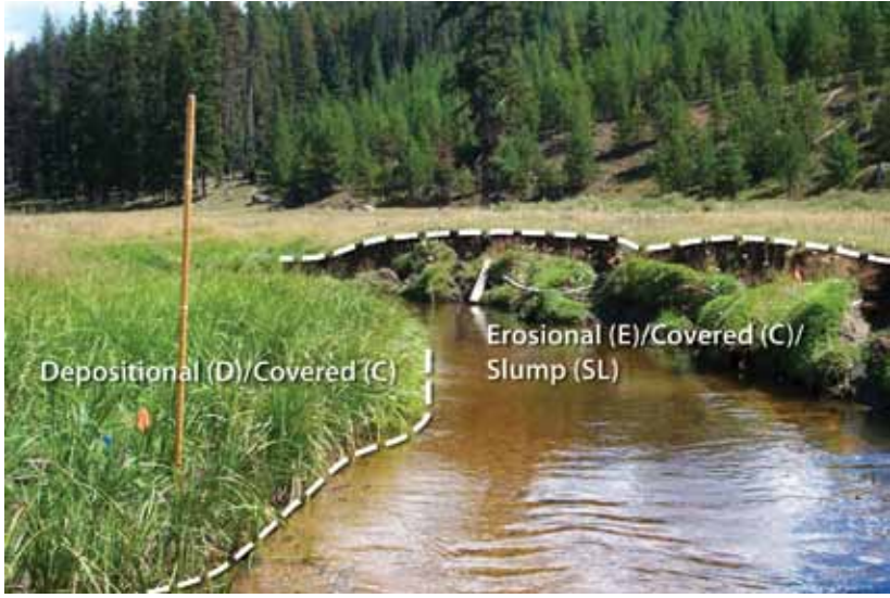
Figure E7. The left streambank is a point bar that is depositional (D) and covered (C). Slump blocks on the right bank are mostly covered with vegetation and are still attached to the streambank above the scour line and therefore are recorded as erosional (E), covered (C), and slump (S). The dashed line is the greenline. Photo - PIBO, U.S. Forest Service.
