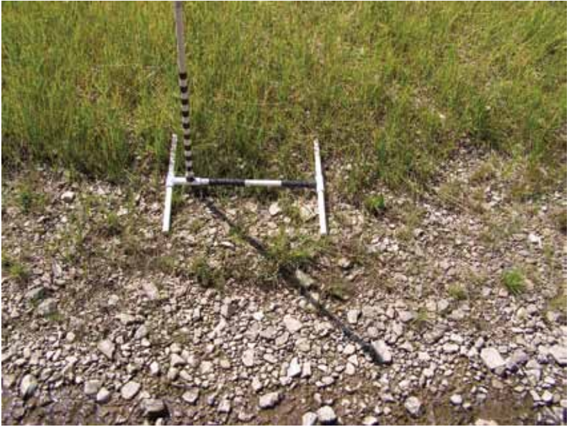
Figure A9. Frequently the greenline is near the bankfull stage. The greenline is located upslope of vegetation closer to the waterline because that vegetation has less than 25 percent foliar cover.
