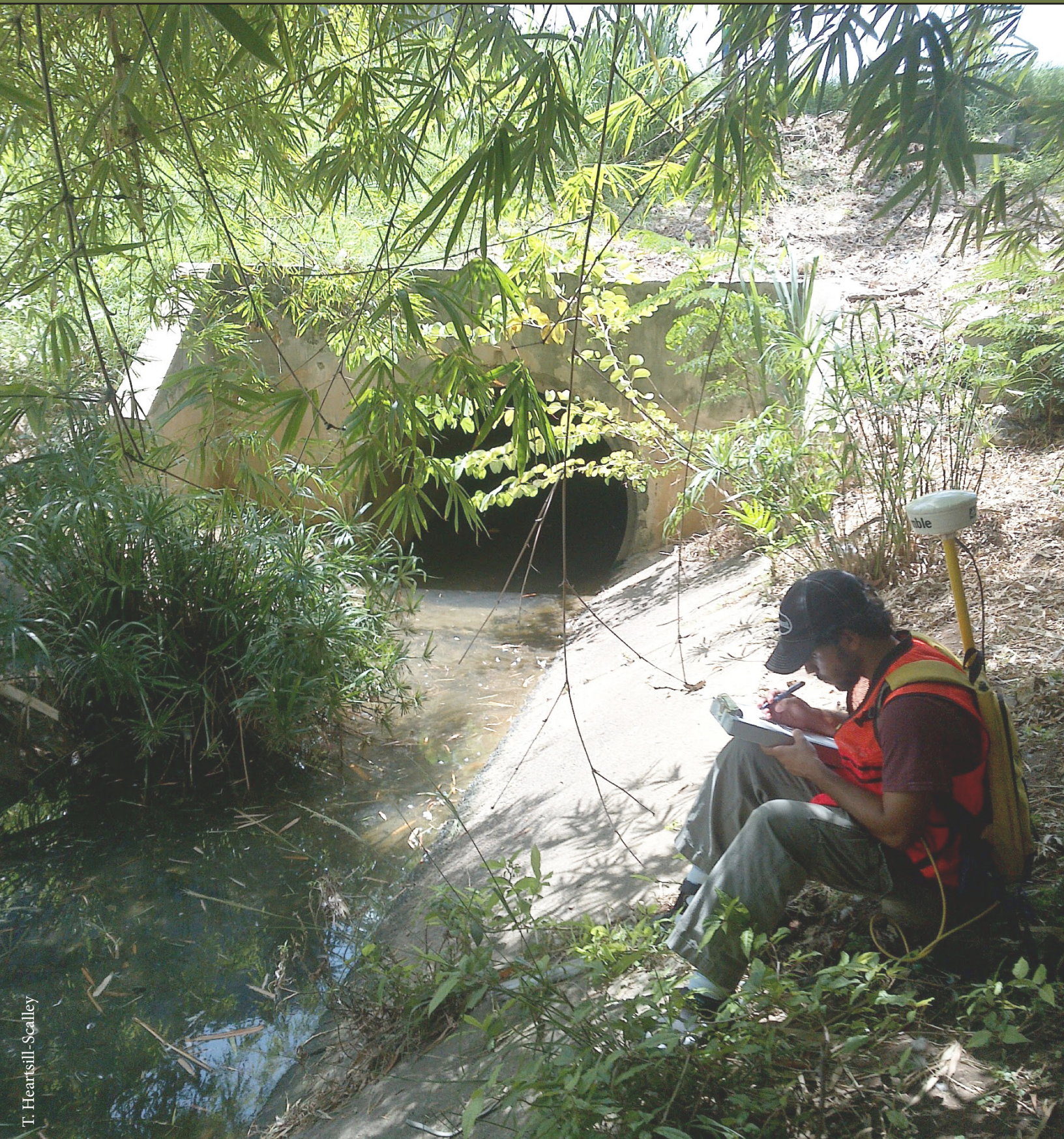
Assessment of a stream reach that combines open channelization with built-up, impermeable (gray) riparian areas and canopy forming vegetation (green) riparian with permeable surfaces.
