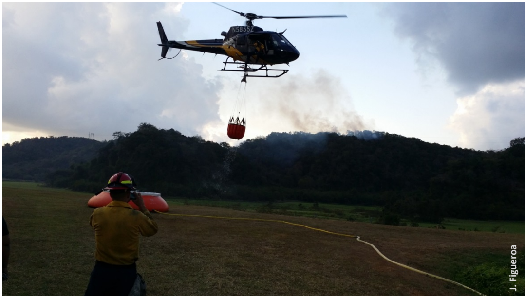
The portable water tank, called a “pumpkin tank” by fire fighters is used to provide water for aerial assault of wild fires. The PR Fire Department holds periodic training as safety is key concern for ground and helicopter crews
