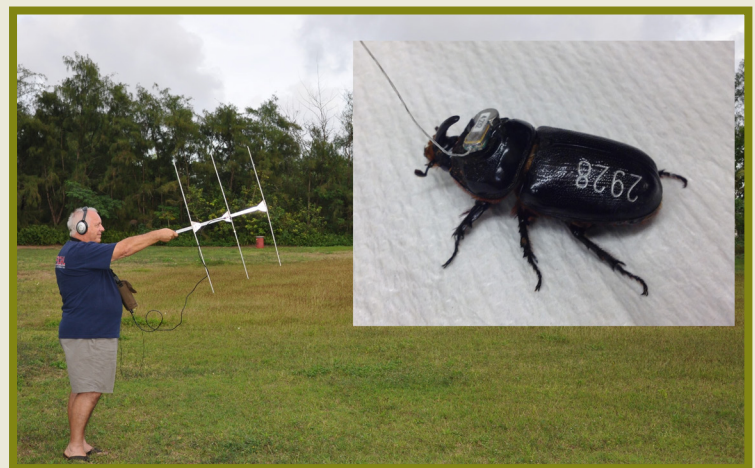
Figure 2. Radio-tracking receiver and coconut rhinoceros beetle with transmitter glued to pronotum.
