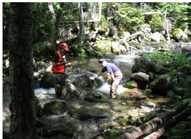
Water temperature logger installation. WMNF photo by Erica Roberts.
