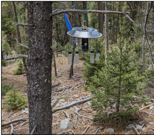
Figure 38: A motorized, rotating spore trap used to monitor airborne spores of Cronartium ribicola , the cause of white pine blister rust; spores are intercepted on microscope slides coated with petroleum jelly and quantified weekly using qPCR.
