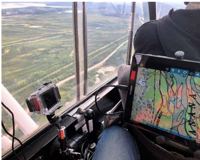
Figure 64 | Damage area polygons are drawn on a digital 1:63,000 USGS quadrangle map. USDA Forest Service photo by Garret Dubois.
