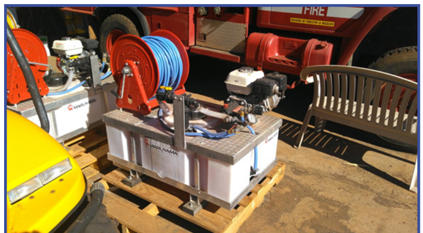
Figure 6. Fifty-gallon sprayer tanks used for invasive species and firebreak treatments (x2). Photo credit: DOFAW
