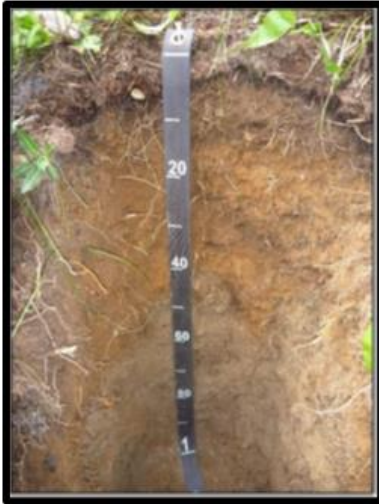
An example of a volcanic ash capped soil. The brightly colored ash can be seen in the horizon between 15–50 cm
