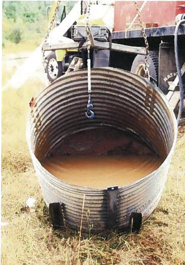
Figure 12. Sediment tank being tipped over for sediment sampling. Note the L shaped tipper bars supporting the tank
