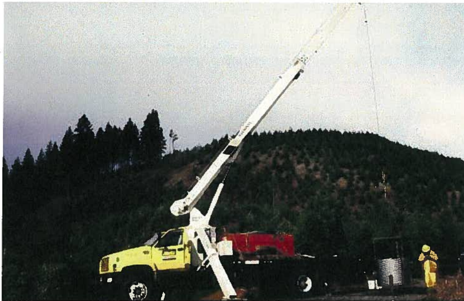
Figure 8. Crane and load cell system used to weigh large sediment samples. Water supply tank is mounted on the bed of the crane
