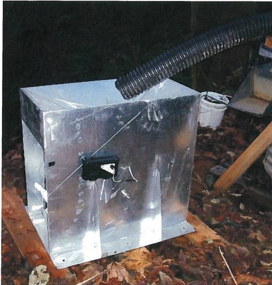
Figure 19. Large free standing tipping bucket with pipe directing flow to inlet.
