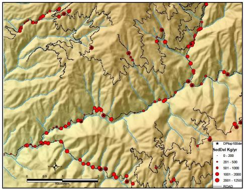
*Figure 2.* Sediment delivery from drain points in Anderson Creek. The red circles are scaled to illustrate sediment delivery. Black stars indicate the location of the top 100 sediment delivery points in the MFP watershed.
