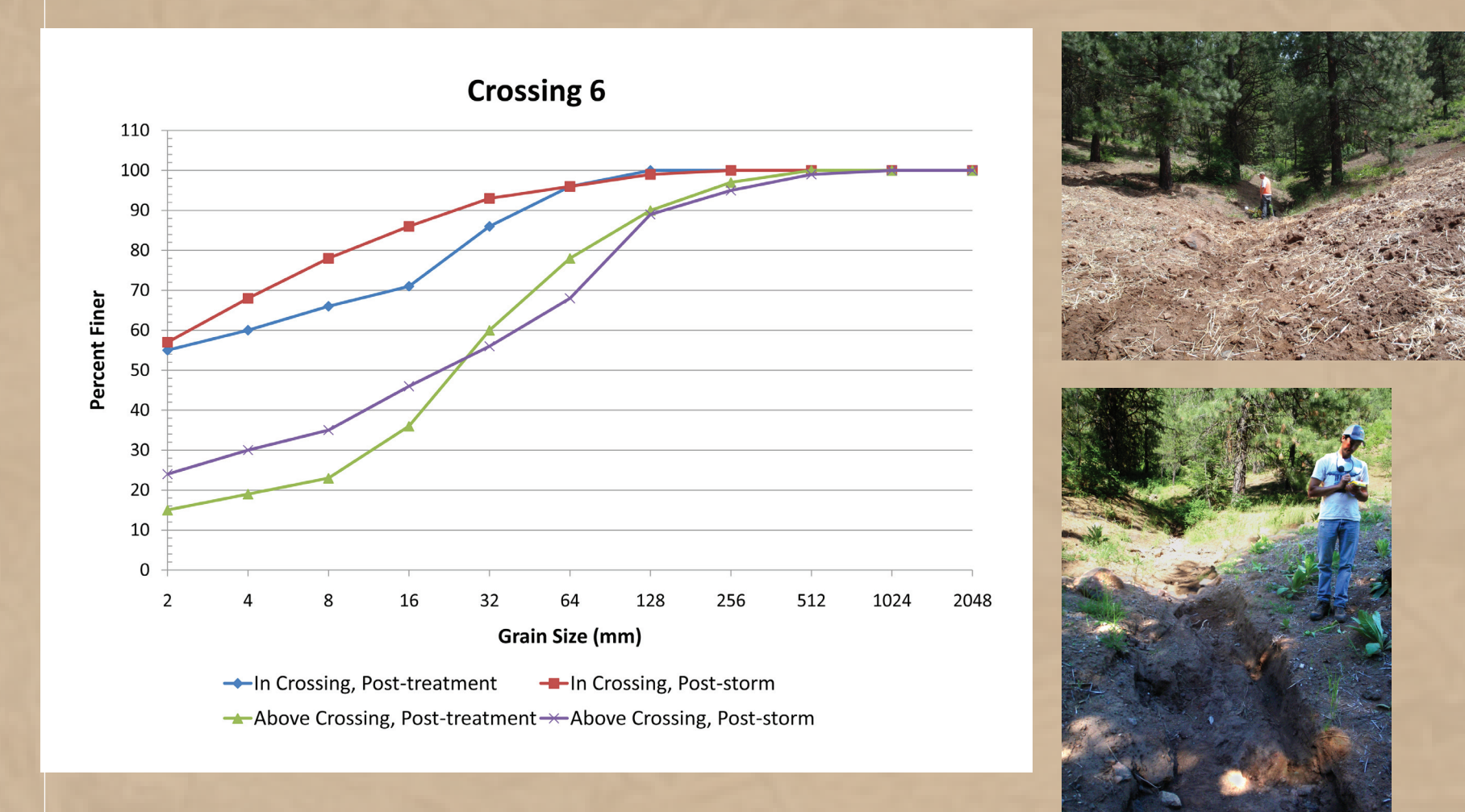
Figure 4. Grain sizes by % for a large stream crossing. Photo before treatment (top) and after treatment (bottom).
