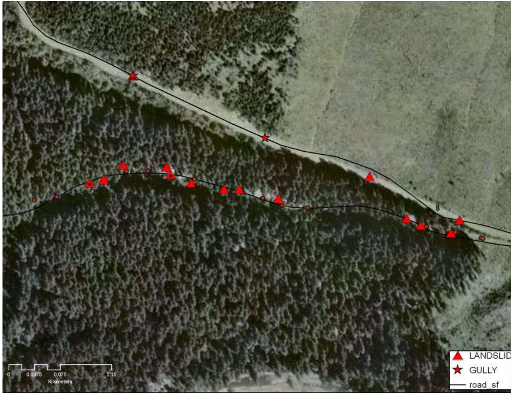
Figure 4. Landslide locations on road 2355-100. These were caused by several upslope roads that routed water and sediment through gullies.
