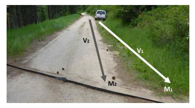
A typical road erosion plot on the Idaho Batholith with two flow paths producing masses  $M_1$  and  $M_2$ .  $V_1$  represents the fraction of the length with vegetation cover on the inside ditch.  $V_2$  represents the fraction of the length with vegetation cover on flow path two, the road surface. In this example V1 has nearly 100% cover so the value is >25% and gets the value .14. The road surface has no live or rooted veg so it is less than 25% and gets a value of 1.
