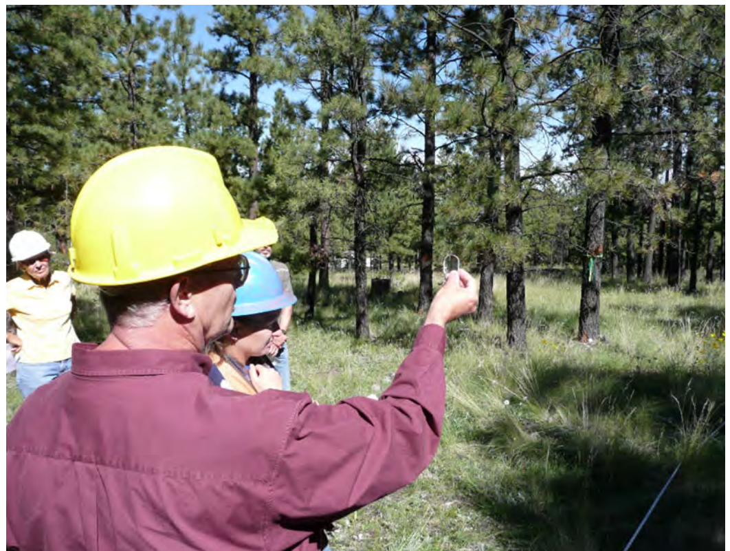
Calculating basal area with prism
