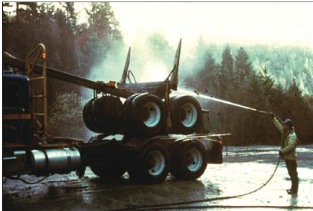
Figure 10.9—Washing a log truck to remove soil potentially infested with Phytophthora lateralis
