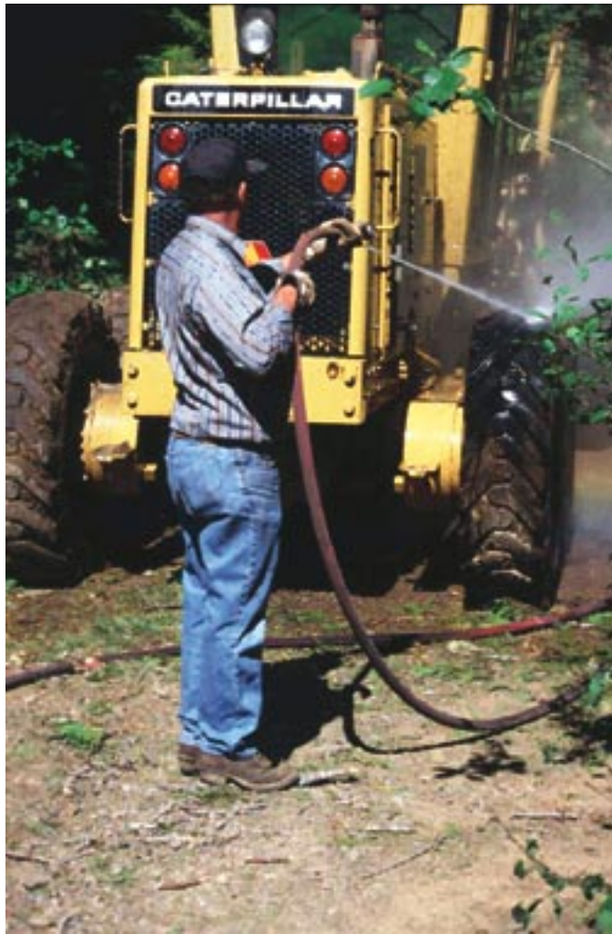
Figure 10.8—Washing equipment to remove soil potentially infested with Phytophthora lateralis
