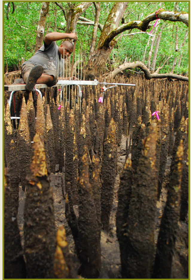
Figure 15. Omekrael Sadang reads a rod surface elevation table in Palau, 2013. (Source: R. MacKenzie)
