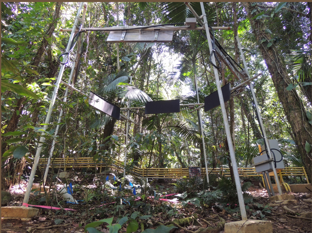
TRACE research plot with associated power lines and control panel in the background. Photo credit: T. Wood.
