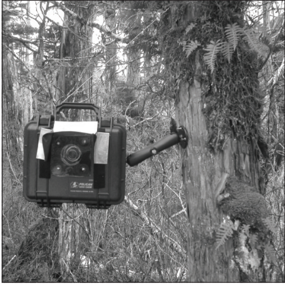
Figure 6—Left, automated snow camera used to record daily snow depths. Right, healthy cedar forest surrounding a bog at 240m elevation with snow covering the ground in April. Snow typically occurs at this site until April or May, often several months after snow melt in the lower elevation dead yellow-cedar forests in the same watershed.
